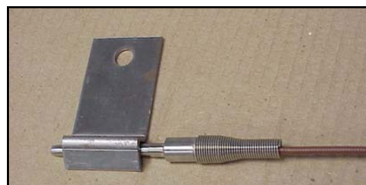
SMC clip with RTD sensor
